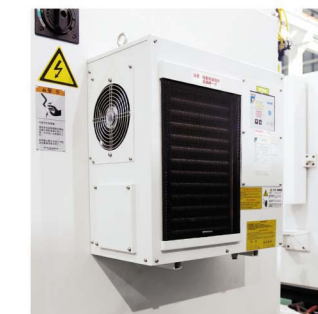
A/C for electrical cabinet
