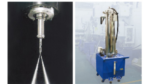
Coolant through spindle (C.T.S) - optional (αT8 motor only)
